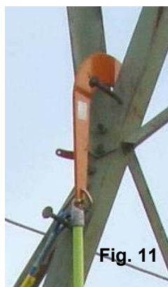
b. Insert rope into channel of Fall Arrester
