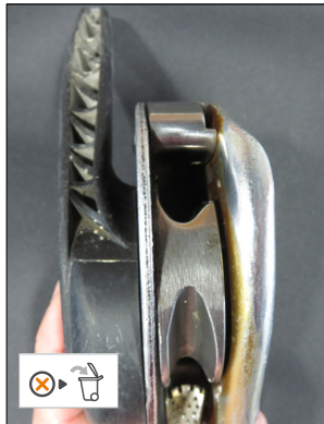
• Worn cam groove
