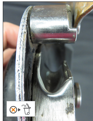
• Cam groove worn to wear indicator
