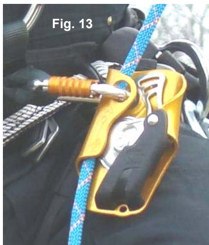
c. Attach carabiner to Fall Arrester
