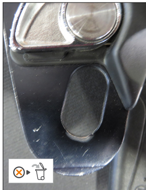
• Attachment hole deformed by a shock load
