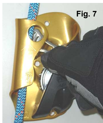
b. Insert rope into channel of Fall Arrester
